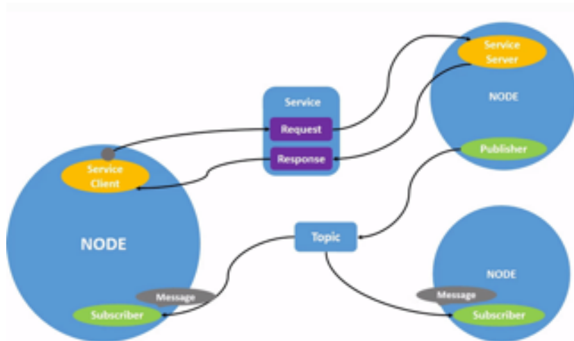
FIGURE 3.7: ROS messaging system runs user code on nodes and provides topics and services for communication [49].
