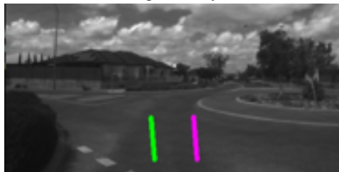
(B) Lane Following Ground Truth (green) vs Model Output (purple) - Round About
