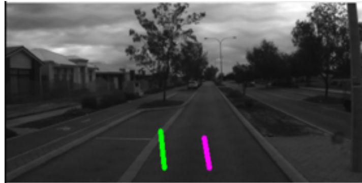
(B) Pull in Ground Truth (green) vs Model Output (purple)
