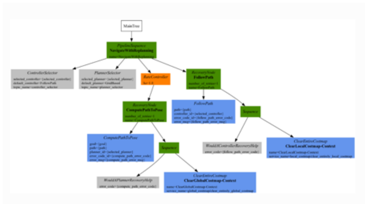
FIGURE 3.10: Example of a navigation behaviour tree in NAV2 [52].
