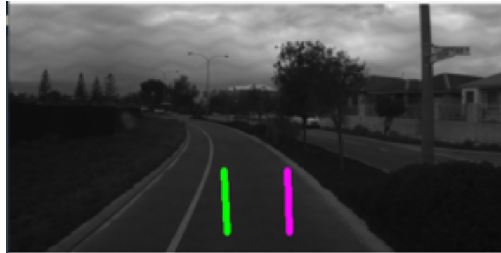
(B) Lane Follow Ground Truth (green) vs Model Output (purple) - Bending Road
