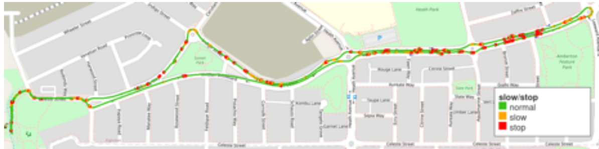
FIGURE 8.16: Slow-stop activations for the Joint LiDAR–Vision model.
