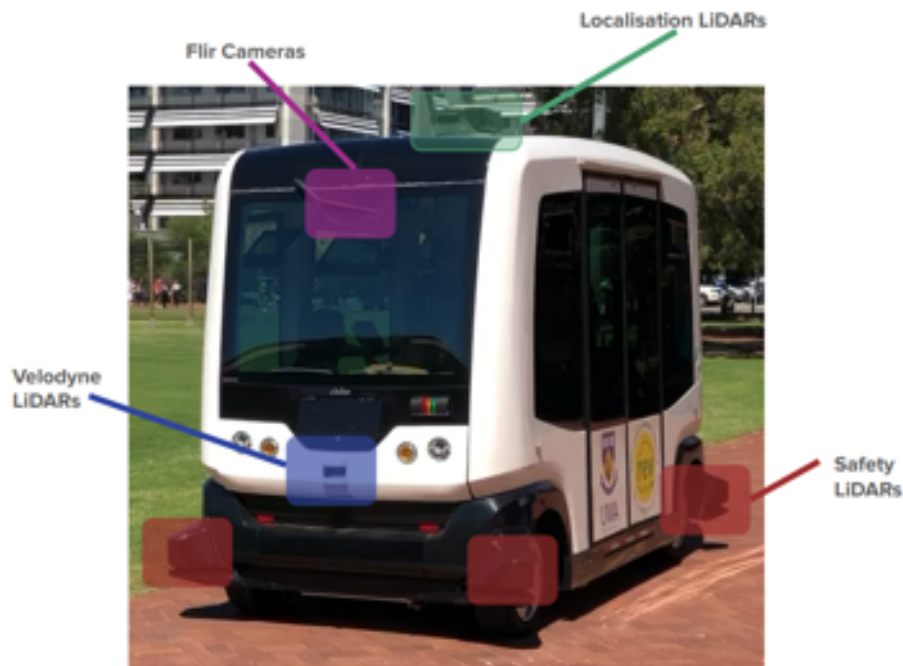
FIGURE 2.5: Autonomous shuttle bus sensor locations.
