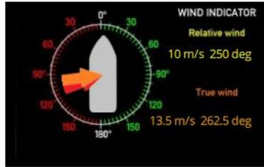
Figure 8 Design of Wind Indicator
