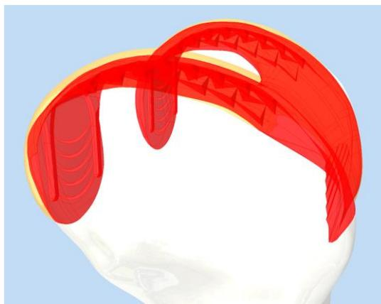
*Figure 5-1: Intersection of femoral implant and femur in Autodesk Inventor.*
