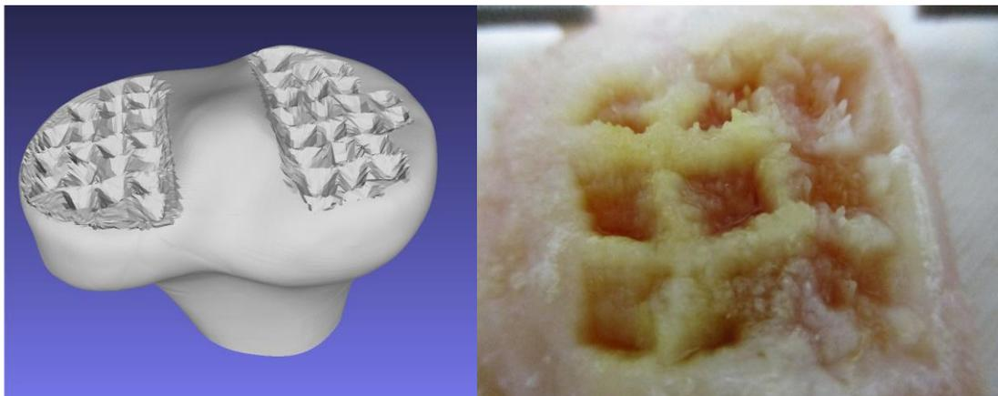
Figure 9-23: Simulated ablated tibia (left), real ablated bone (right).
