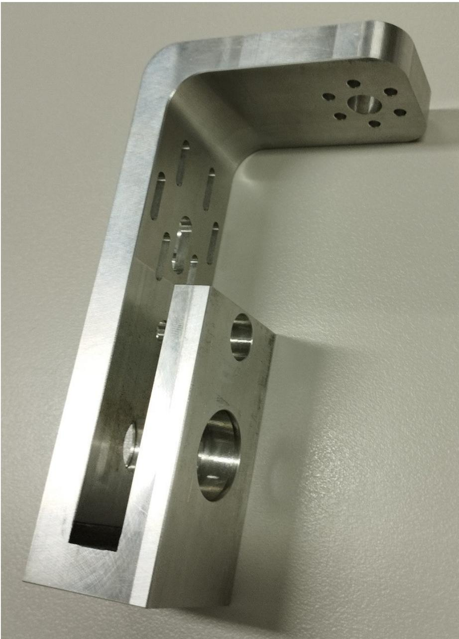
**Figure 27:** *One of the six wheel mounts.*
