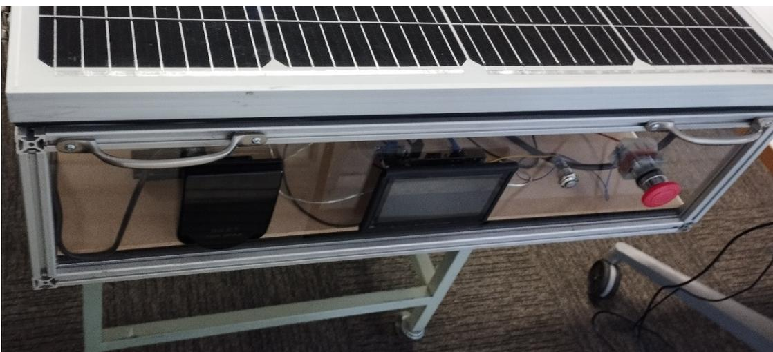
**Figure 23:** View of the back of the rover with the Raspberry Pi screen, buttons and charging plug mounted.
