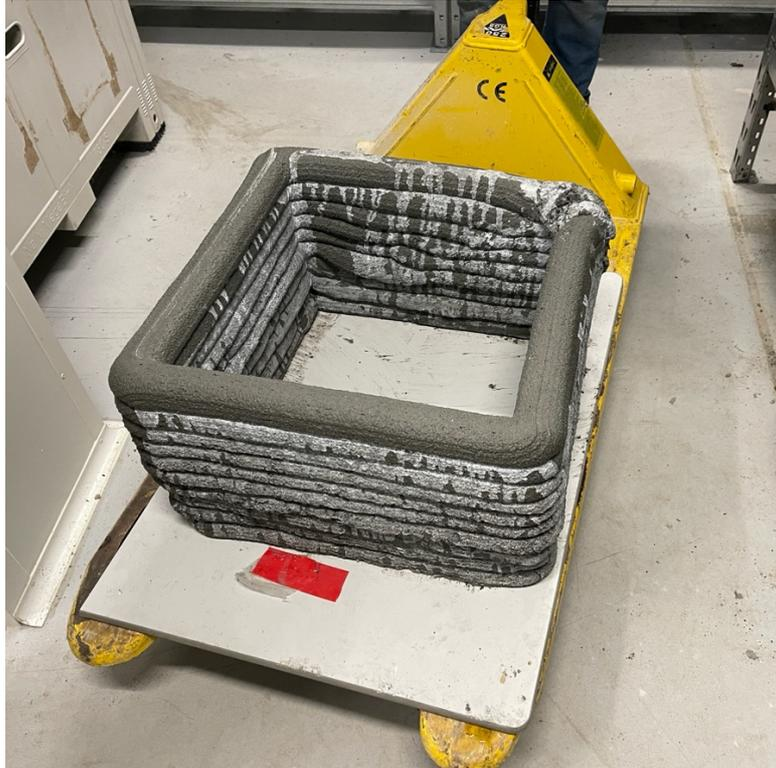
**Figure 21 Final Concrete 3D Print with the Nachi robotics manipulator.** After many attempts and overcoming challenges, the “Concrete 3D Printing” project were successful.
