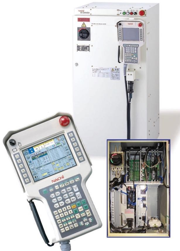
**Figure 2 Nachi AX20 Controller with the Teach Pendant (“Nachi Controller”).** Nachi Controller is used to provide power to the robot and to control every aspect of the robotic manipulator. Nachi Controller have the following functions: manual control, software limits, program creation, program conversion, program execution, IO signals, etc...
