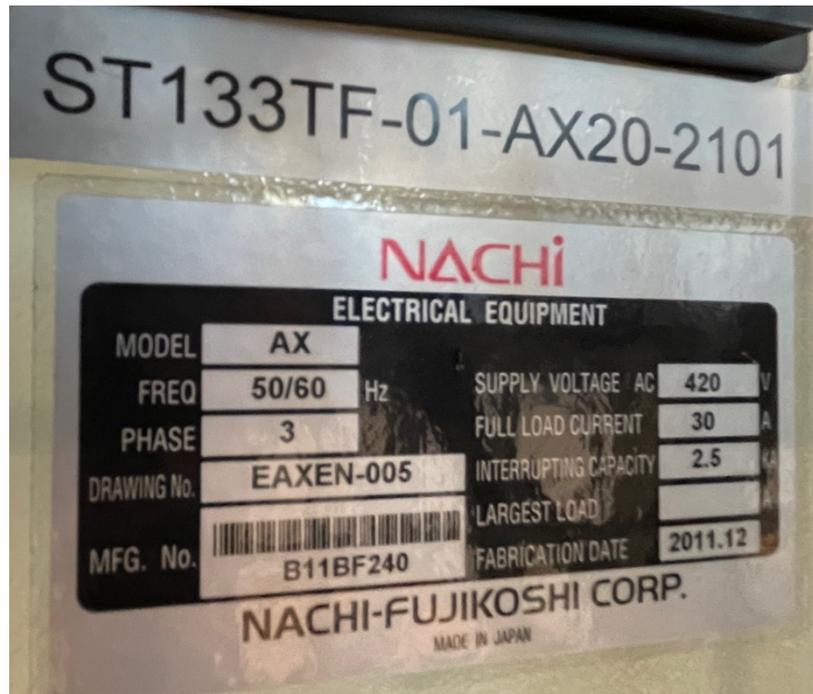
**Figure 7 Power specification and Nachi Controller's model number.** Nachi system (Nachi and Controller) runs on 3-phase, 420 volts and 30 amps of current.
