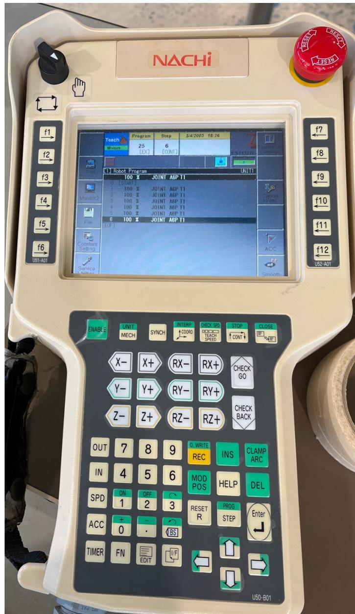
**Figure 8 NACHI Controller's Teach Pendant.** It's the main point of communication for the manual and automatic control of the NACHI robotics manipulator. It enables writing, testing, and execution of all programs. Display shows Program #25 and Step #6 is highlighted (in focus).
