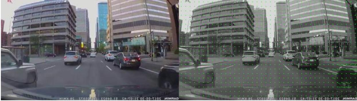
Figure 4 Camera image (left), optical flow grayscale image (right)<sup>1</sup>
