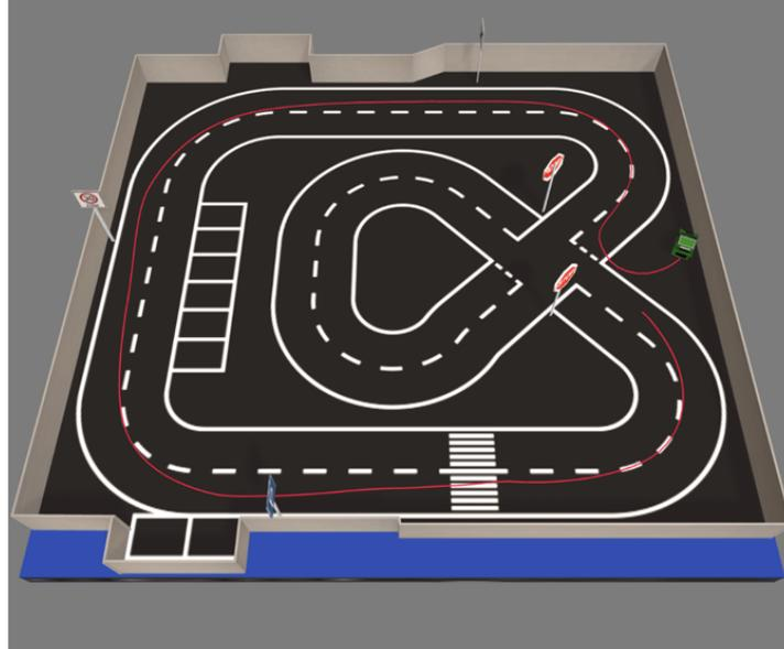
Figure A.6: Path taken by CNN trained Autonomous robot with 3000 images and no data repetition
