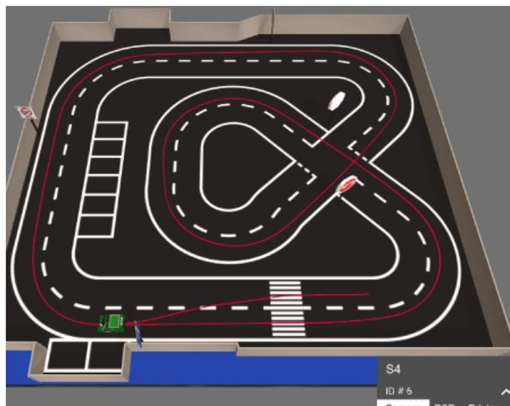
Figure A.7: Successful lane detection with ROF
