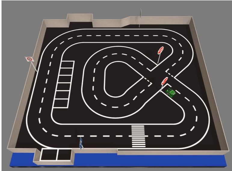
**Figure 3.2:** *EyeSim simulation environment with road signs, lane markings and driving robot*
