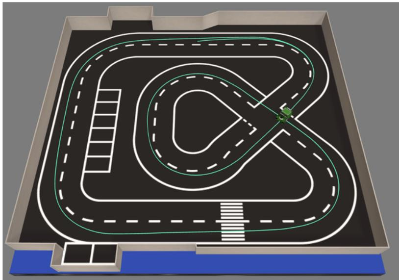
Figure A.3: *Path taken by CNN trained Autonomous robot in EyeSim within the same training environment*
