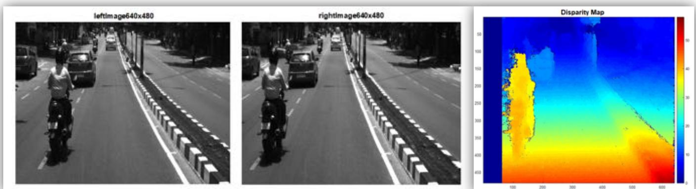
**Figure 12 - Example of SGBM generated stereo disparity map [30]**
