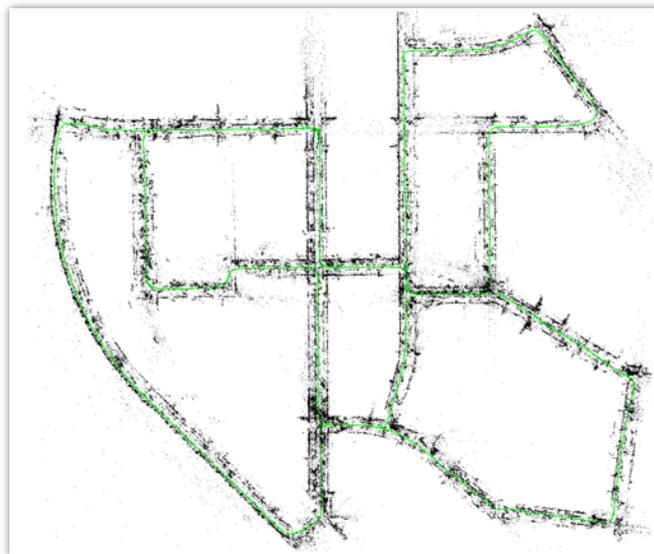
**Figure 7 - ORB SLAM2 Trajectory and Environment Reconstruction, with loop closures [22]**
