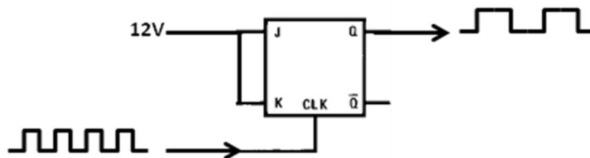
**Figure 3.7 - JK flip flop, frequency divided by 2 feature**
