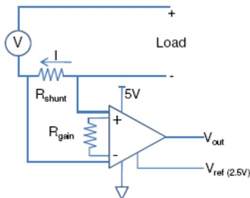
**Figure 3.4 - A current sensor**
