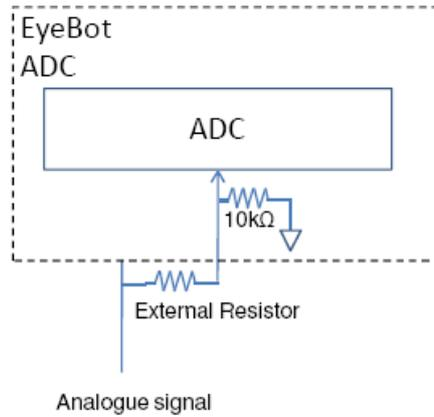
**Figure 3.2 - Simplification of the ADC voltage division capacity**
