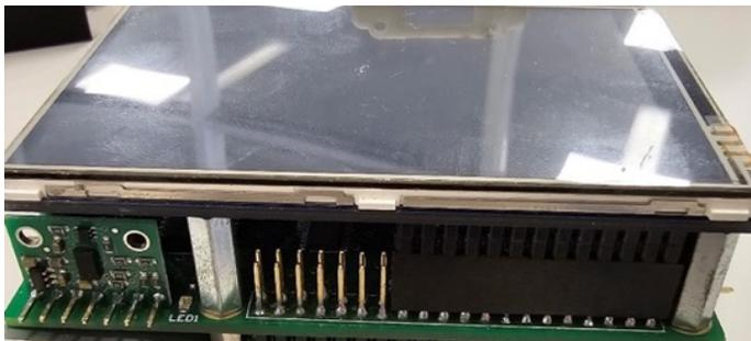
Figure 4.12. LCD Screen Connected to IO-Board
