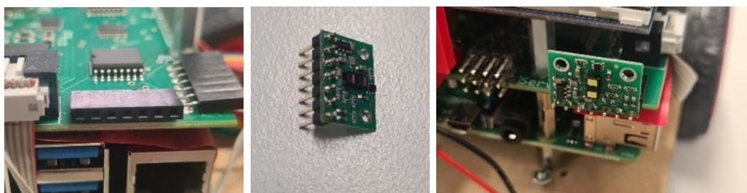
Figure 4.11: PSD Sensor socket (left). PSD Sensor (middle). connected PSD Sensor (right)
