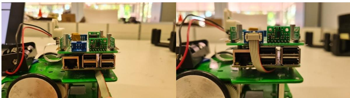
Figure 4.9: Motor port without (left) and with (right) motor connected.
